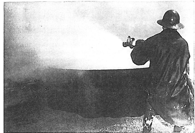
Single 1½-in. all-purpose nozzle projecting high-velocity fog cone, delivery volume approximately 54 gpm, used to extinguish No. 2 fuel oil in 10-ft. diameter tank.
